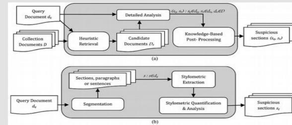
Fig. 1. Framework for different plagiarism detection systems. (a) White-box design for extrinsic plagiarism detection system. (b) White-box design for intrinsic plagiarism detection system.
